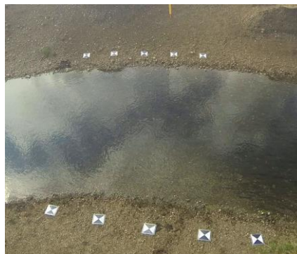
Figure 9. Uncorrected barrel distortion which creates curvature in what are actually straight lines. Typically occurs in wide angled lens (Source: Sophie Pearce, Newcastle University, UK).
