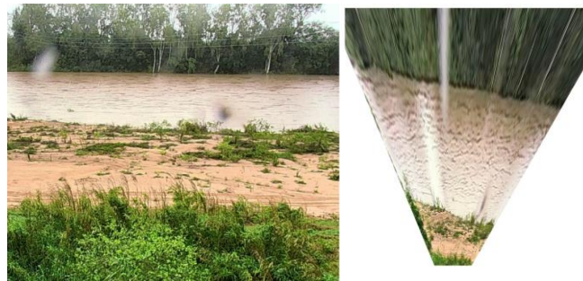
Figure 17. Oblique camera image (left), and the rectified image adjusted for increasing pixel ground size as distance from the camera increases. Source: Mark Randall, RDMW, using HydroSTIV software.
