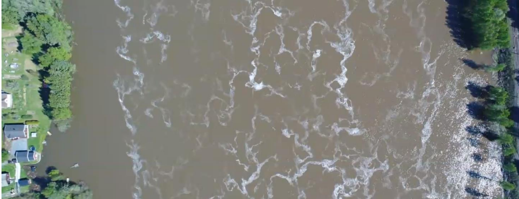
Figure 8. An image from a drone flood video in Norway. Tracer particles that are advected with the flow are clearly visible across most of the channel width. This video is very good for image velocimetry analysis. Source: Kristoffer Florag-Dybvik, Norwegian Water Resources and Energy Directorate (NVE).
