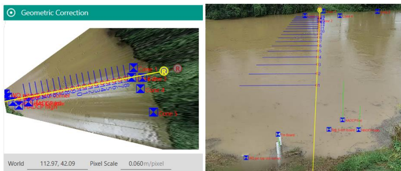
Figure 11. An orthorectified image (Left) based on the real-world coordinates of each ground control point and the original camera image (Right). Source: Mark Randall, RDMW, using HydroSTIV software.
