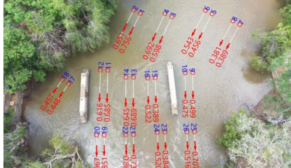
Figure 5. Multiple STIV search lines undertaking velocity analyses along a short channel reach. Source: Mark Randall, RDMW, using HydroSTIV software.
