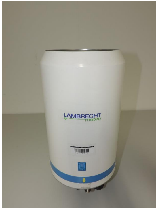
assembled rain gauge
