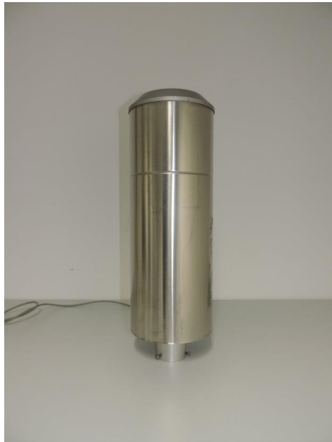
assembled rain gauge
