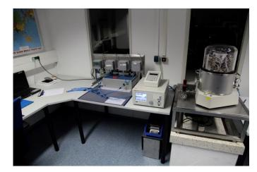
Examples: calibration with a pressure balance (left) and calibration with a pressure controller and standard (down)
