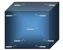
To evaluate inhomogeneity, thermometers are typically placed in corners of calibration area and one in the geometrical centre.
