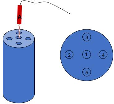
**Stability**: Reading of the thermometer in one of the wells ( $L_{A1}$ ) for a time t
