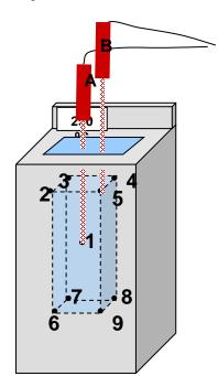
Temperature measurements in the 8 positions of the figure and in the central point.
