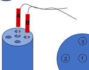
For not calibrated thermometers, we have to find the relative correction the thermometers. For doing this, the thermometers interchanged between two wells:
