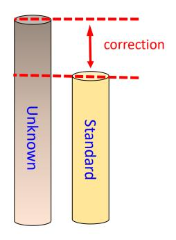
Correction = Standard – reading of instrument under calibration
