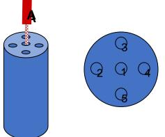
**Stability**: Reading of the thermometer in one of the wells ( $L_{A1}$ ) for a time t
