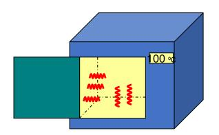
Measurements of temperature with thermometers with different emissivity. The thermometer with lower emissivity will give the closest value to real air temperature inside the climate chamber
