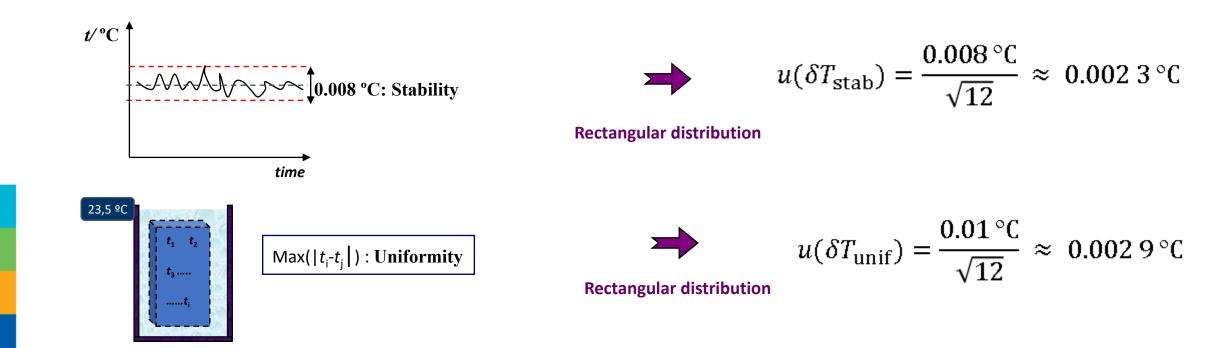
$$u^2(T_{\text{ref}}) = u^2(\delta T_{\text{s,cal}}) + u^2(\delta T_{\text{s,drift}}) + u^2(\delta T_{\text{s,read}}) + u^2(\delta T_{\text{stab}}) + u^2(\delta T_{\text{unif}})$$
