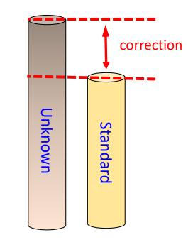
Correction = value of Standard – reading of instrument under calibration
