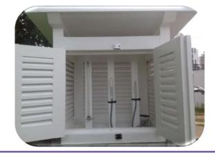
Many sensors are mounted inside other infrastructure, for example temperature/humidity sensors are typically installed in a screen. In this case, the infrastructure needs to meet the Operating Conditions.
