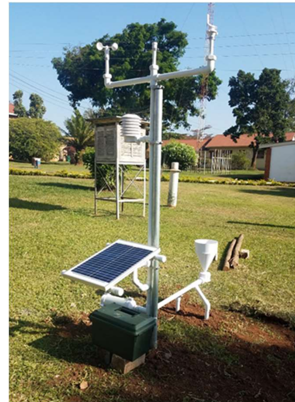
Example: 3D-Printed Automatic Weather Station (3D-PAWS)
