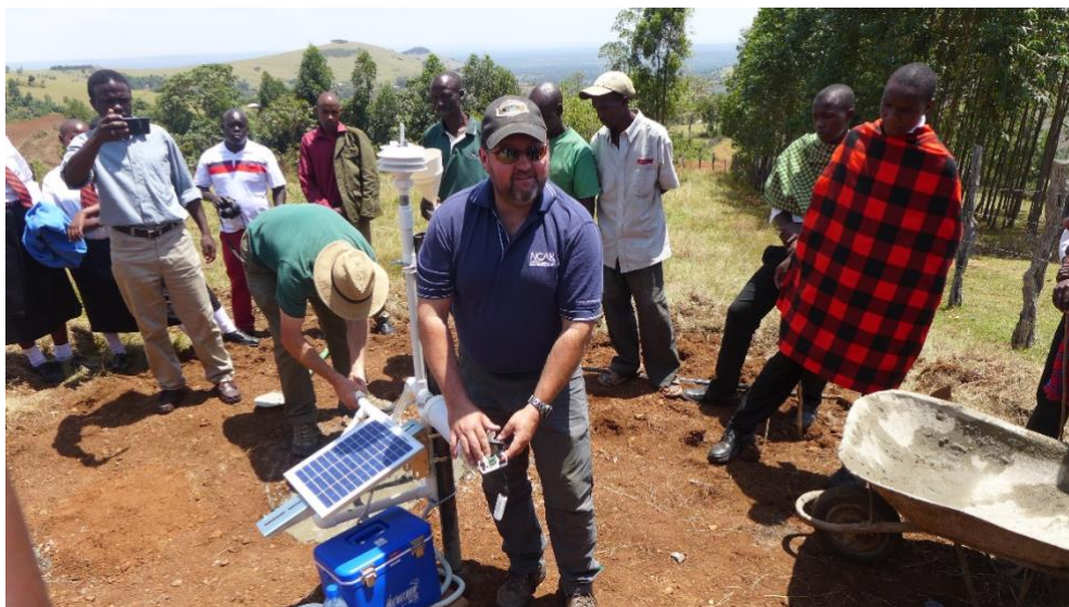
Figure 16.1. Paul Kucera explaining the instrumentation included in a 3D-PAWS at Sirua Aulo Secondary School in Kenya.
