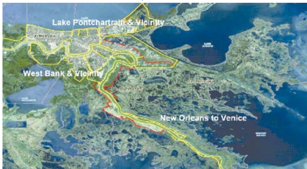
Figure 4.1 Three USACE Hurricane Protection Systems in Southeast Louisiana
