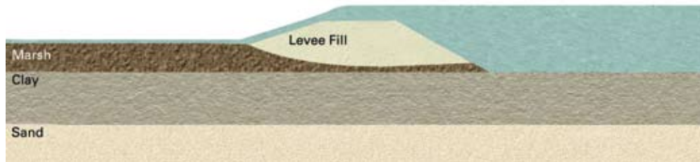
Figure 7.10 Overtopped Levee Erosion Failure Mechanism
