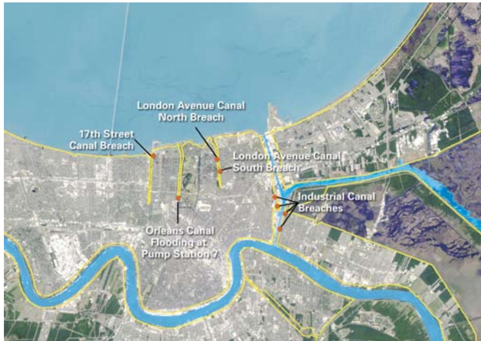
Figure 5.3 Major Breaches in the New Orleans Hurricane Protection System
