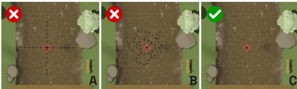
Figure 18: Schematic representation of UAV movement during video recording with a perpendicular view. (A) Longitudinal and/or transverse displacements. (B) Large erratic movements. (C) Stable or with minimal movement over a fixed position.
