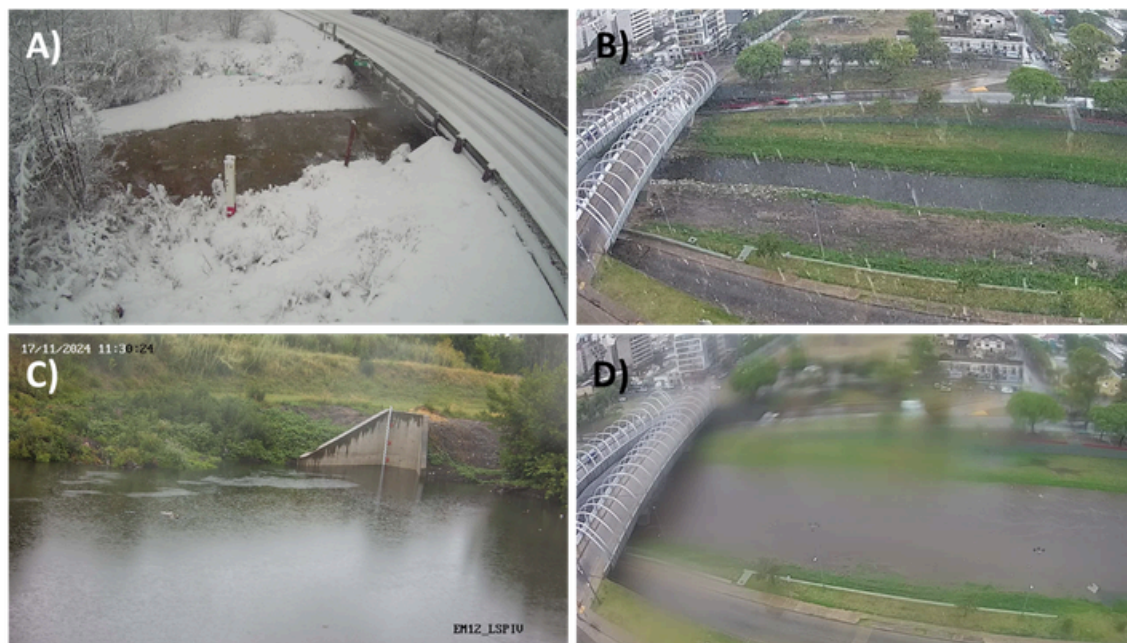
Figure A.4.16: Examples of recordings during precipitation events. A) Visibility of snowflakes. B) Visibility of raindrops. C) Deformation of the water surface due to raindrop impact. D) Camera lens wet from rain. Source: Own elaboration. Some images were provided by the National Hydrological Service of Environment and Climate Change Canada
