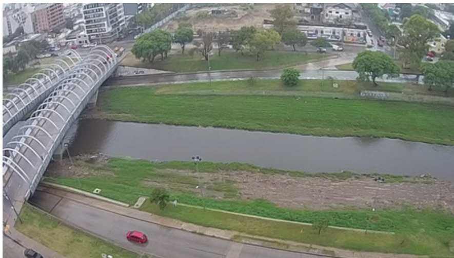
Figure A.4.10: Example of tracers not being visible due to the recording point being too far from the flow. Source: Own elaboration
