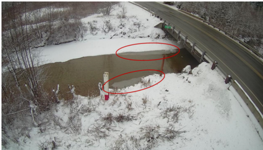
Figure A.4.17: Static ice sheets on the flow surface. Source: Image provided by the National Hydrological Service of Environment and Climate Change Canada
