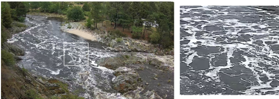
Figure A.4.2: Example of surface foam as a natural surface tracer. Source: Own elaboration
