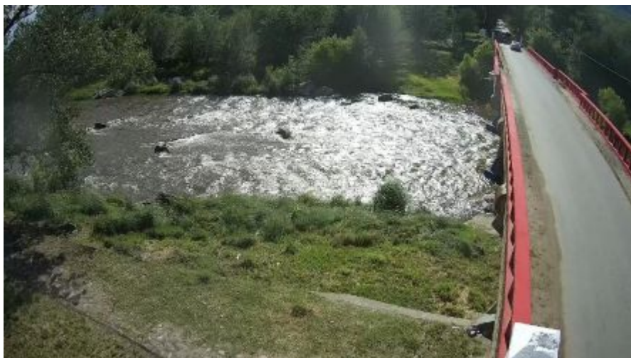
Figure A.4.13: Presence of undesired sun reflections over the flow measurement area. Source: Own elaboration
