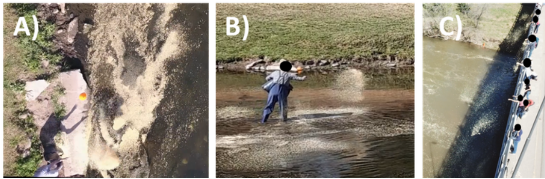
Figure A.4.8: Examples of seeding methods. A) From the riverbanks. B) From within the channel. C) From a structure (bridge) crossing the channel. Source: Own elaboration
