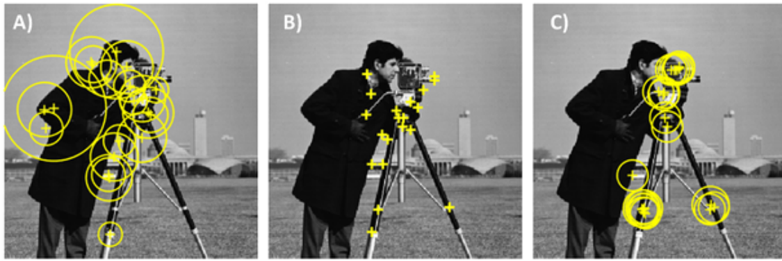
Figure A.1.2: Examples of feature detection algorithm applications. A) SURF, B) FAST, C) ORB. Source: Own elaboration
