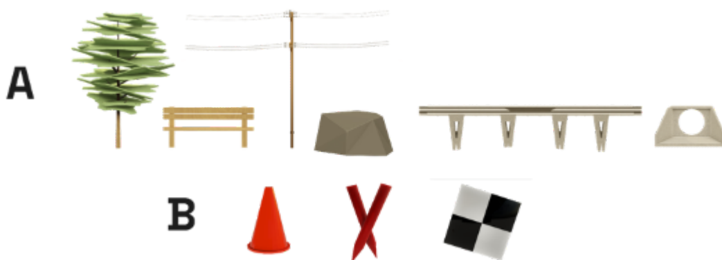
Figure 30: Examples of elements that can be used as CPs. (A) Pre-existing elements found at the site. (B) Examples of temporary markers. Source: Own elaboration
