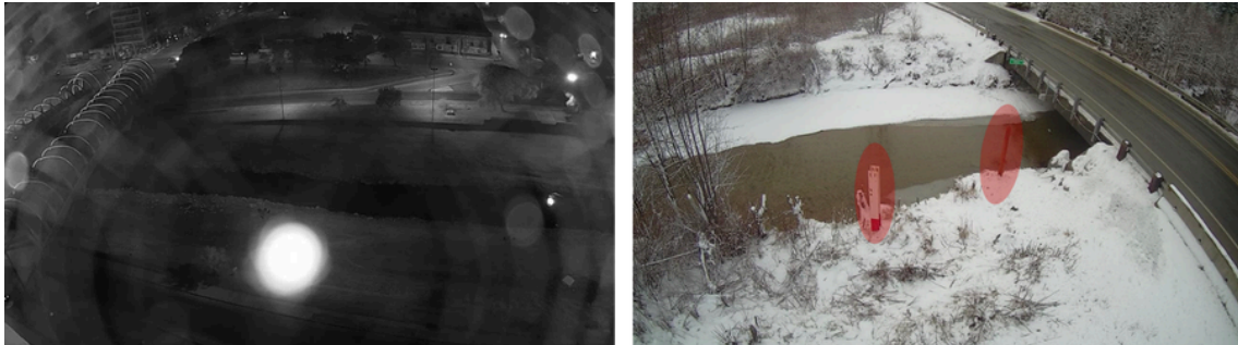
Figure A.4.11: Elements obstructing the view of the flow measurement area. Left: Insect on the camera lens. Right: Objects at the site partially obstructing the flow. Source: Own elaboration. Some images were provided by the National Hydrological Service of Environment and Climate Change Canada
