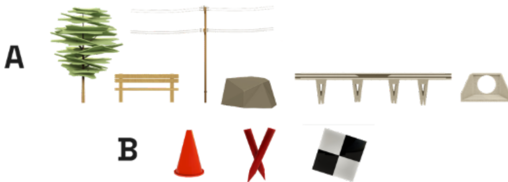
Figure 22: Examples of elements that can be used as CPs. (A) Pre-existing elements found at the site. (B) Examples of temporary markers. Source: Own elaboration
