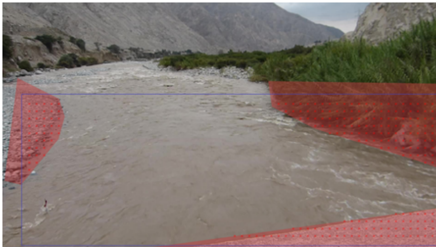
Figure 47: Definition of the Region of Interest (ROI) and masks. The ROI is represented by the blue rectangle, while the masked areas are shown in red. Source: Own elaboration
