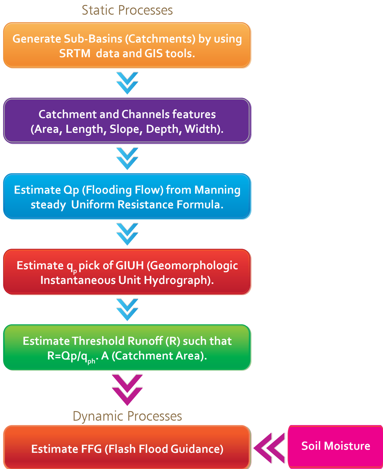
Figure-54 BSMEFFG hydrologic processes flowchart
