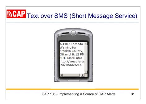
"Smart phones" can receive full CAP alerts. For other cellular telephones, the Short Message Service (SMS) provides a way to receive text alerts that originated as CAP. The CAP "headline" element is specifically designed to be sent over SMS.
